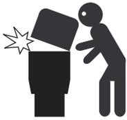
**NEVER** operate the filter system at more than 50 psi of pressure. Operating the filter system in excess of 50 psi can cause product failure or also cause the filter lid to be blown off, which can cause death, serious personal injury or property damage.
