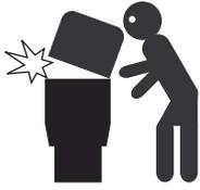
**NEVER** start pump while standing within five (5) feet of the filter. Starting the pump while there is pressurized air in the system can cause product failure or also cause the filter lid to be blown off, which can cause death, serious personal injury or property damage.
