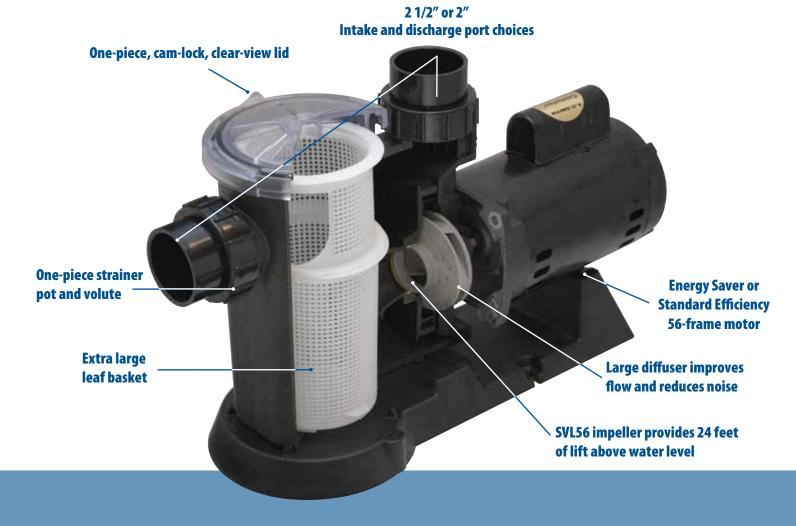
SVL56 Pumps are available in Energy Efficient and High-Flow Models.
