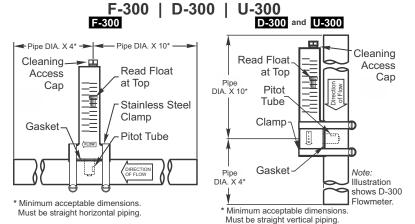
**General:** Flowmeter should only be used on the schedule 40 IPS (ASTM-D-1785) size and type of pipe for which it is intended. Incorrect use will result in inaccurate readings and leakage problems.
