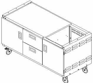
2.Place the grill head on the top of trolley with 6 piece of 1/4"x 1/2" screws. Make sure 6 screws are tightening. **Note: Remove four handles from inside side shelf to outside.**Then assemble two side shelves by using 8 piece of M5 Hex-Philip bolts. (Four for each side shelf)
