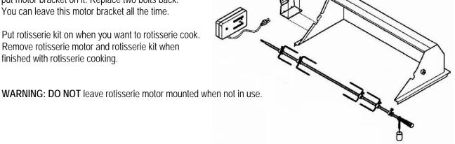
5. Place the rotisserie rod in the door storage when finished with rotisserie cooking.
