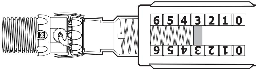
If necessary, use the valves in the pool equipment area to adjust the flow so that the red indicator is at the Number 3 setting.
