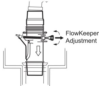
If the pool has more than one (1) skimmer, connect the hose to the one (1) closest to the pump.
