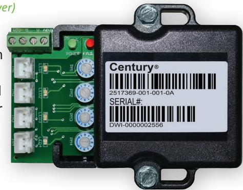
Contents include — automation adapter (shown), digital input cable, lead cable, RS-485 connector, conduit fitting, terminal box cover assembly, plugs, screw driver, and instructions.
