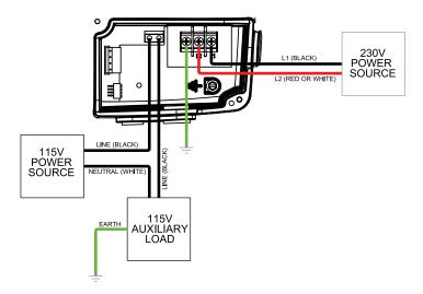
Figure 2: Wiring Diagram with 115V Aux Load
