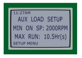
The Auxiliary Load is a relay inside the control designed to provide AC power to a load that should not be energized without adequate water flow from the pump (i.e. heater, boost pump, salt water chlorinator).
