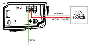
Figure 1: Wiring Diagram without Aux Load
