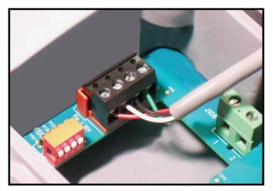
Figure 14: UI connector installed
