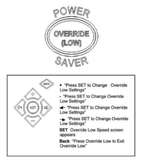
**NOTE:** Press + to increase the speed. If the value is at 3450, the screen reads "Maximum Speed for this Motor is 3450 RPM." If the fourth digit is flashing, press + and the speed increases by 5.
