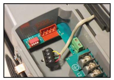
Figure 13: Communication Connector Removed
