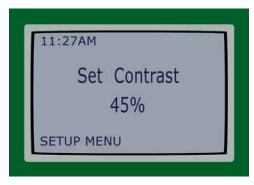
This menu will change the contrast of the LCD screen to optimize viewing for various lighting conditions.
