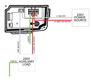
Figure 3: Wiring Diagram with 230V Aux Load
