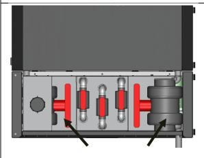
03. Unscrew the outside collars of the 3" (80mm) ball valves. Place the sheetmetal valve covers over the 3" plubing lines.
