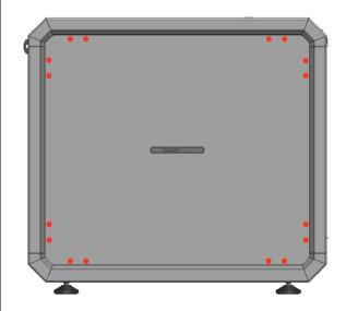
03. To access the electronics module internals remove the cover panel by unscrewing the 16 M5 cap head screws with the 4mm hex key provided.
