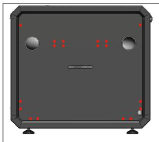
01. Remove the two plumbing end sheetmetal cover panels by unscrewing the 18 M5 cap head screws with the 4mm hex key provided.
