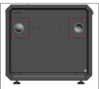
02. Remove the two sheetmetal valve covers by unscrewing the 8 M4 nuts with a 7mm (9/32") socket.
