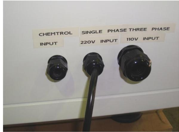
02. Electrical Inputs from left to right. ORP input, Single phase input, Three phase input.
