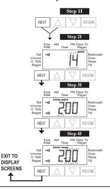
**Step 1I -** To enter Installer Display press the NEXT and ▲ buttons simultaneously for five seconds and release.
