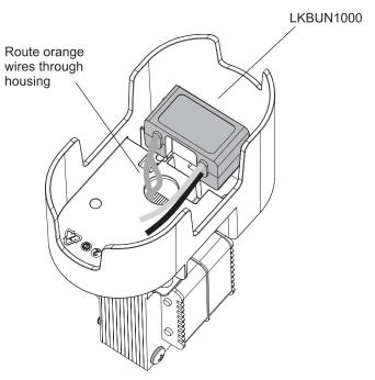
Insert the LKBUN1000 as shown. Push down until it locks then route the orange wires through the hole in the housing.
