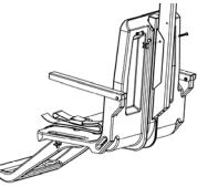
18. Attach foot rest to seat with bolts and thumbnuts.
