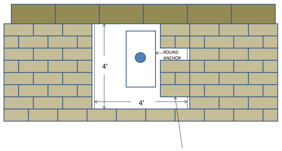
**Option #2** same as Option 1, just recess the concrete down and reinstall the pavers over the concrete except directly under the lift, That section needs to be concrete
