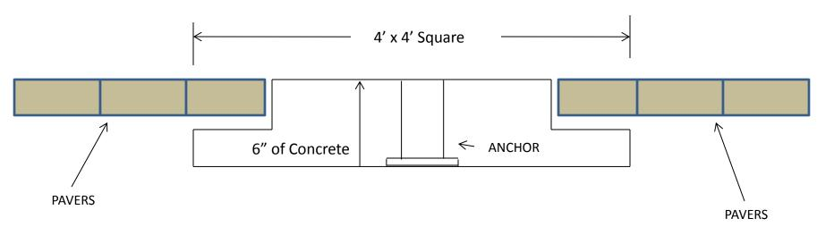
**Option #2** same as Option 1, just recess the concrete down and reinstall the pavers over the concrete except directly under the pool lift, That section needs to remain concrete!
