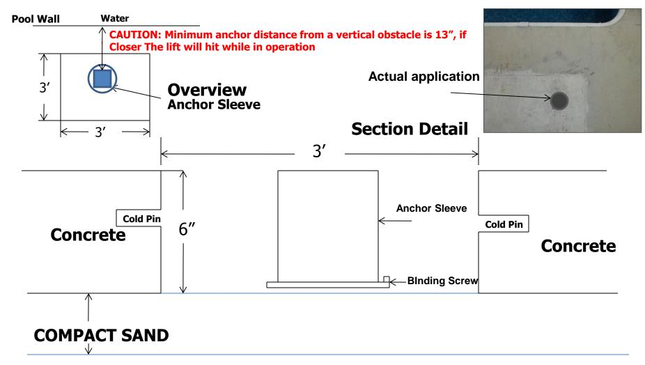
Front of Anchor Sleeve must be 12" to 36" from the water's edge or 13" min if an obstacle is present before the water. Connect the binding screw to your bonding grid
