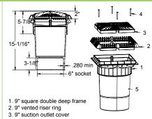
4. 10 x 1-3/4" flat head phillips type-a screw, 316 ss 5. 6" socket deep pvc sump
