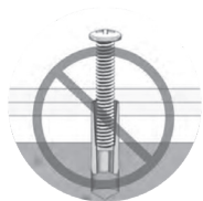
FIGURE 2 IF SCREW HOLE HAS DAMAGED THREADS
