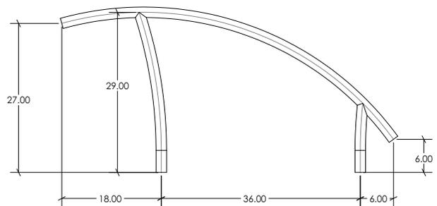
Note: Leg lengths on all Artisan rails include 4" to go into anchors.
