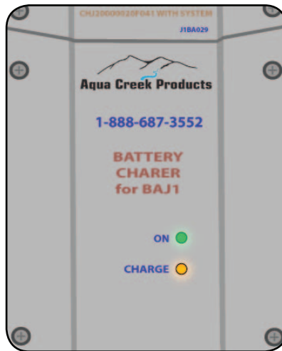
The Battery is CHARGING when the orange light is glowing
