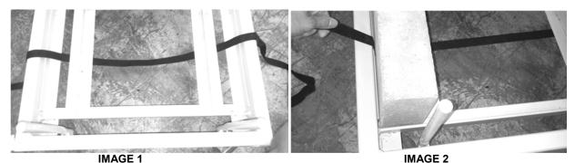
Lace the belts through the frame, as shown in **image 1**. Place the outer most blocks in position, as shown in **image 2** and pull the slack out of the restraint belts.
