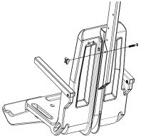
27. Attach foot rest to seat with bolts and thumbnuts.
