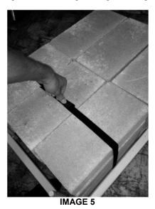
Tighten both straps as shown in Image 5 across the top of both rows of weights. Loop the strap through its buckle and pull firmly securing each top row of weights.
