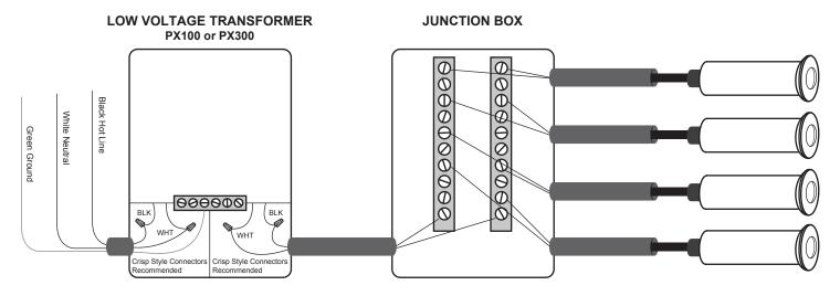
**NOTE:** This Diagram is to be used as a guide line only for a typical System Installation and should only be used as such. It is the Installers sole responsibility to verify and assure that proper gauging of secondary wiring from the Transformer to the J-Box are in compliance with your local, State and National Electrical Codes.
