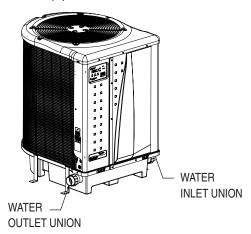
**Heat Pump Water Connections**
