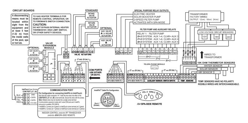
IntelliTouch/EasyTouch Load Center Wiring Diagram
