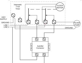
AutoSet Contactor to Mechanical Timer Wiring Example
