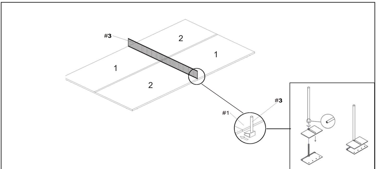
*NOTE: If tennis table is used over billiard table it is recommended that the EVA support block be placed under the center of the table tennis surface for extra support.*
