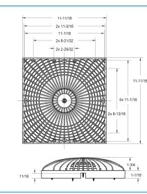
Designed to replace off-standard 12" square covers that fit into mud frames that are 1" deep
