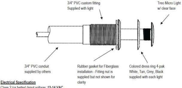
Class 2 (or better) Input voltage: 12-14 VAC Color Change (RGB): 1.5 Watts max.
