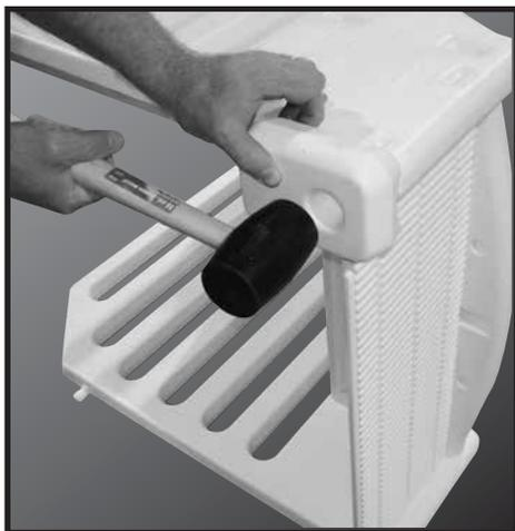
**#7:** Position a foot pad over the round extension located on the bottom of side panel. It will require several hard hits with a rubber mallet to force the foot pad over the extension. Repeat to install the three remaining foot pads. Stand the step upright.
