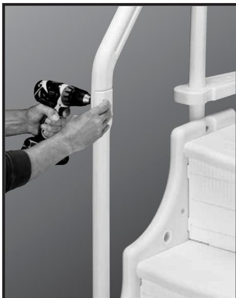
**#6:** Match the indents on one of the handrails with the indents on the rail posts and attach the handrail using two 2-1/2" bolts and two 1/4" x 20 hex nuts.
