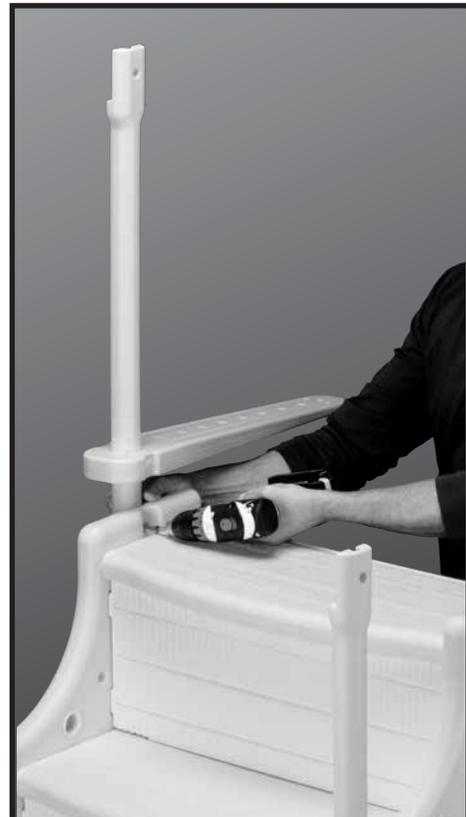
**#4:** Attach the remaining two rail posts to the upper post locations of the side panels by repeating step #1.
