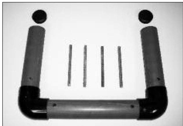
Fig. 2 Plastic Anchor Jig for In Deck Installation
