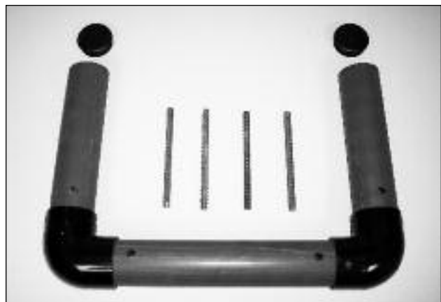
Fig. 2 Plastic Anchor Jig for In Deck Installation
