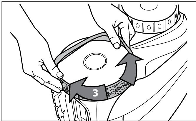
**Figure 39. Work the Tire On Around the Wheel**
