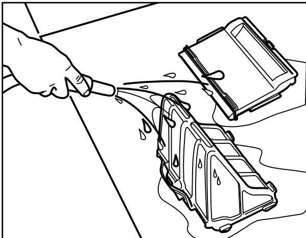
3. Remove filter canister and rinse with clean water. Plug power cord back into control unit and store cleaner for next use.
