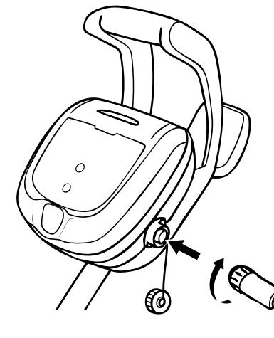
**Figure 13. Connect Power Cable**
