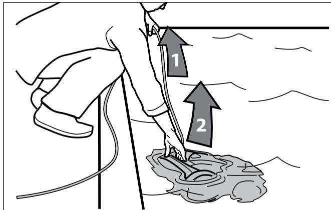
**Figure 18. Remove Cleaner From Pool with handle**
