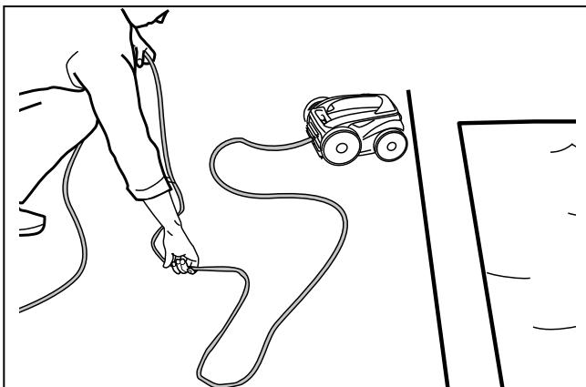
2. Remove the cleaner from the pool and untangle all kinks and coils in the power cable starting at the cleaner head.
