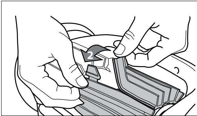
**Figure 31. Undo the Tabs of the Brush**
