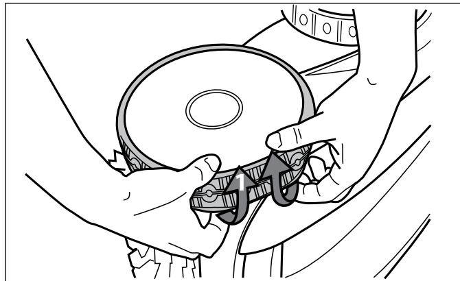
**Figure 35. Pull the Old Tire Over the Wheel**
