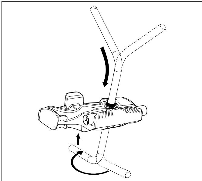
**Figure 3. Connect Metal Frame to Base Unit**
