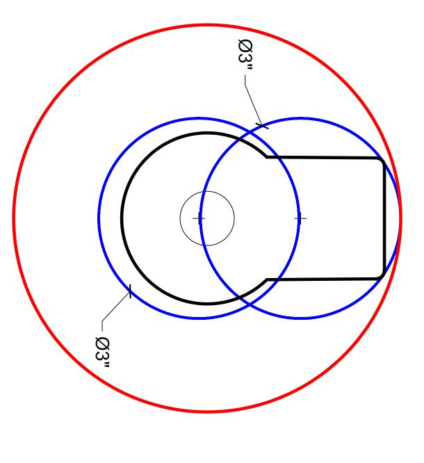
BLUE LINES = 3" Overlapping Core holes drilled to depth of 4-1/2".
