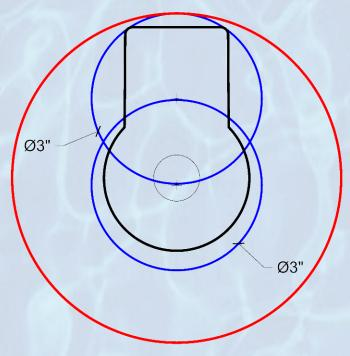
BLUE LINES = 3" Overlapping Core holes drilled to depth of 4-1/2".
