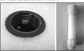
NOTE: This Extension Piece is made up by the installer. It is comprised of 2" MTP (male threaded pipe) Fitting on bottom, 2" FIP for top and a section of 2" PVC pipe cut to the correct size to achieve the desired height.
