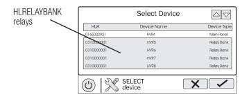
Note that the device name in the relay table corresponds to the following relays on the HLRELAY-BANK:
