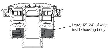
FIGURE 6: EXTRA WIRE IN HOUSING
