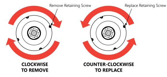
FIGURE 9: LED MODULE INSTALLATION
