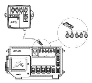
**Note:** Before powering the Aeware spa pack, make sure all accessories are linked to the bonding connector and connected to the spa pack. Make sure that the spa pack door is closed, then turn on the breaker.
