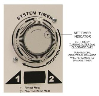
Provides timer control over heating and filtration cycles. To activate a timed cycle push the teeth on the timer outward, each tooth represents 2 hours of operation. The (2) modes of operation are based on the rocker switch under the timer and are as follows:
