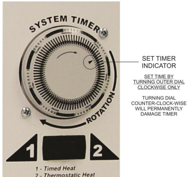
Provides timer control over heating and filtration cycles. To activate a timed cycle push the teeth on the timer outward, each tooth represents 2 hours of operation. The (2) modes of operation are based on the rocker switch under the timer and are as follows:
