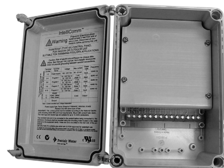
IntelliComm Communication Center
