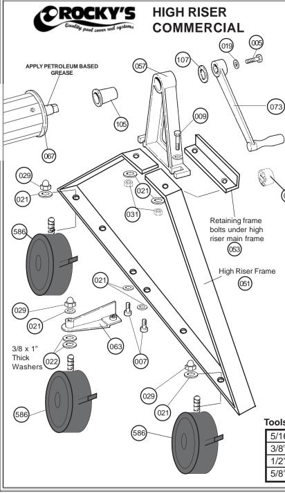
**Important:** Before you start to assemble make sure that the third leg (#063) holes in the High Riser frame are pointing inwards. These holes are nearer to the edge of the frame.
