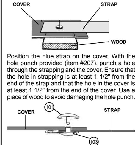
Position the blue strap on the cover. With the hole punch provided (item #207), punch a hole through the strapping and the cover. Ensure that the hole in strapping is at least 1 1/2" from the end of the strap and that the hole in the cover is at least 1 1/2" from the end of the cover. Use a piece of wood to avoid damaging the hole punch.
