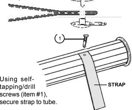
Using self-tapping/drill screws (item #1), secure strap to tube.
