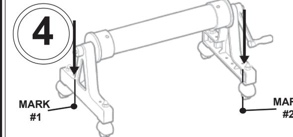
Using one of the two holes in the A-frame as a guide, make mark #1 on deck. With a 1/2" concrete drill bit, drill a 1 1/2" deep hole at mark #1. Complete steps 5 and 6 before continuing with step 4. On the other side of the roller unit, make mark #2 by using one of the two holes in the A-frame as of guide. With a 1/2" concrete drill bit, drill a 1 1/2" deep hole at mark #2.
