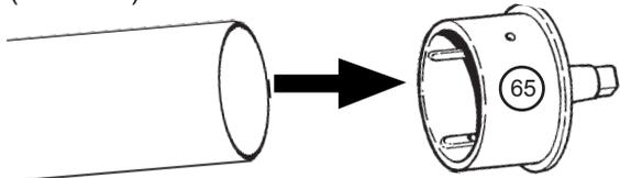
With 2 self-drill/tapping screws (item #1), attach hub to tube using electric drill. Apply pressure to ensure screw cuts into aluminum tube then cuts it's own thread. *(No predrilling required)* **Repeat with other side.**
