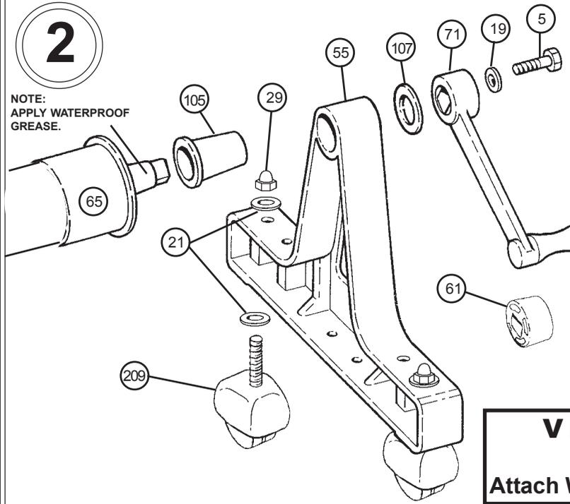
Bolt the castors (item #209) to the A-frames (item #55), as shown in the diagram.
