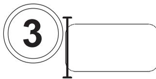
For regular shaped pools, align the outside edge of the tube parallel with the end of the pool.
