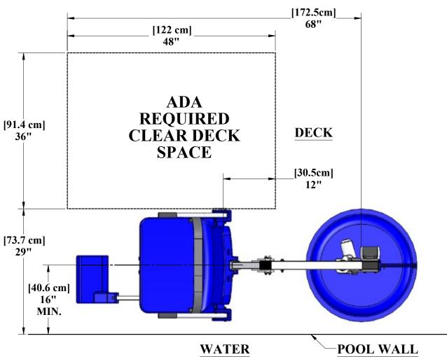
Before installing the Revolution Lift it will be necessary to select a location for the anchor. The Revolution Lifts versatility allows it to be installed in a wide variety of locations, but the owner/installer should be aware of the requirements of the Americans with Disabilities Act (ADA) with concern to lift installations. The diagram above shows an example of an ADA compliant installation, which incorporates the following ADA rules in order to be compliant;
