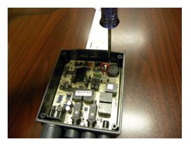
RETURN THE THREE (3) SCREWS TO SECURE THE CONTROL BOARD BACK IN PLACE
