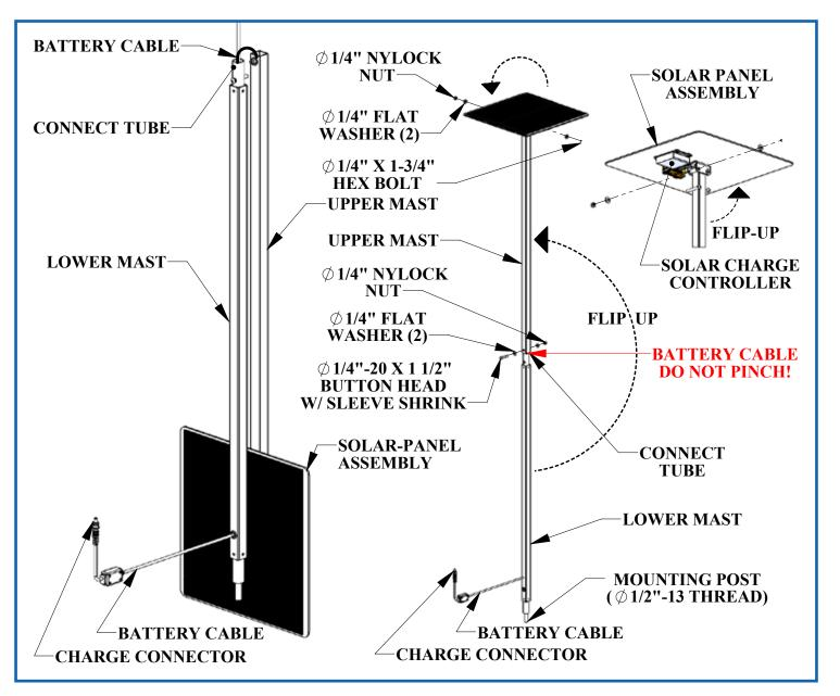
To assemble the Solar Charger you will need two (2) 7/16" wrenches or sockets and a 5/32" allen key.
