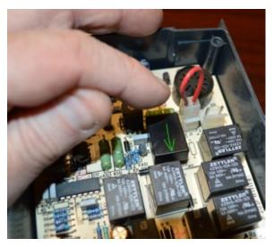
REPLACE THE EMERGENCY-SWITCH CAP WITH "ARROW" POINTING DOWN AS SHOWN
