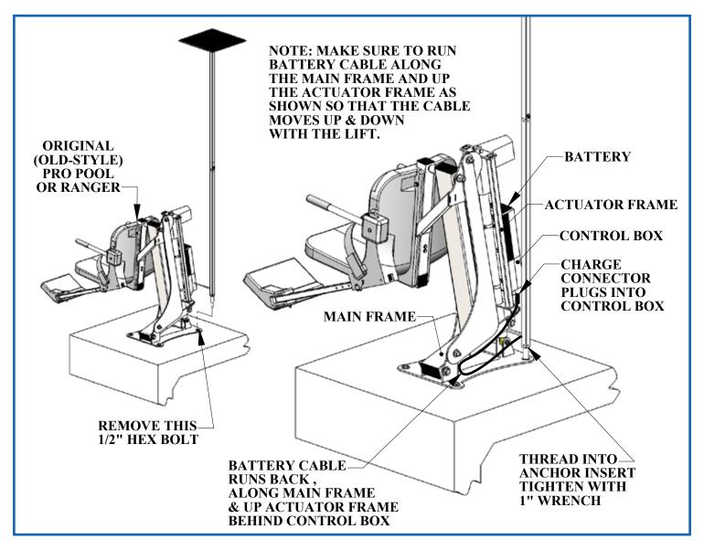
Installing the Solar Charger on an original-style Pro Pool/Ranger Lift;
