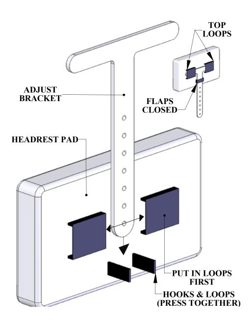
The ADJUST BRACKET must be removed from the assembly to install or remove the HEADREST PAD. When installing the pad thread the bracket through the middle loop first and slide the pad up to the top loops. Thread the bracket through the top loops (one at a time) to complete the installation. To remove the pad, reverse this procedure.
