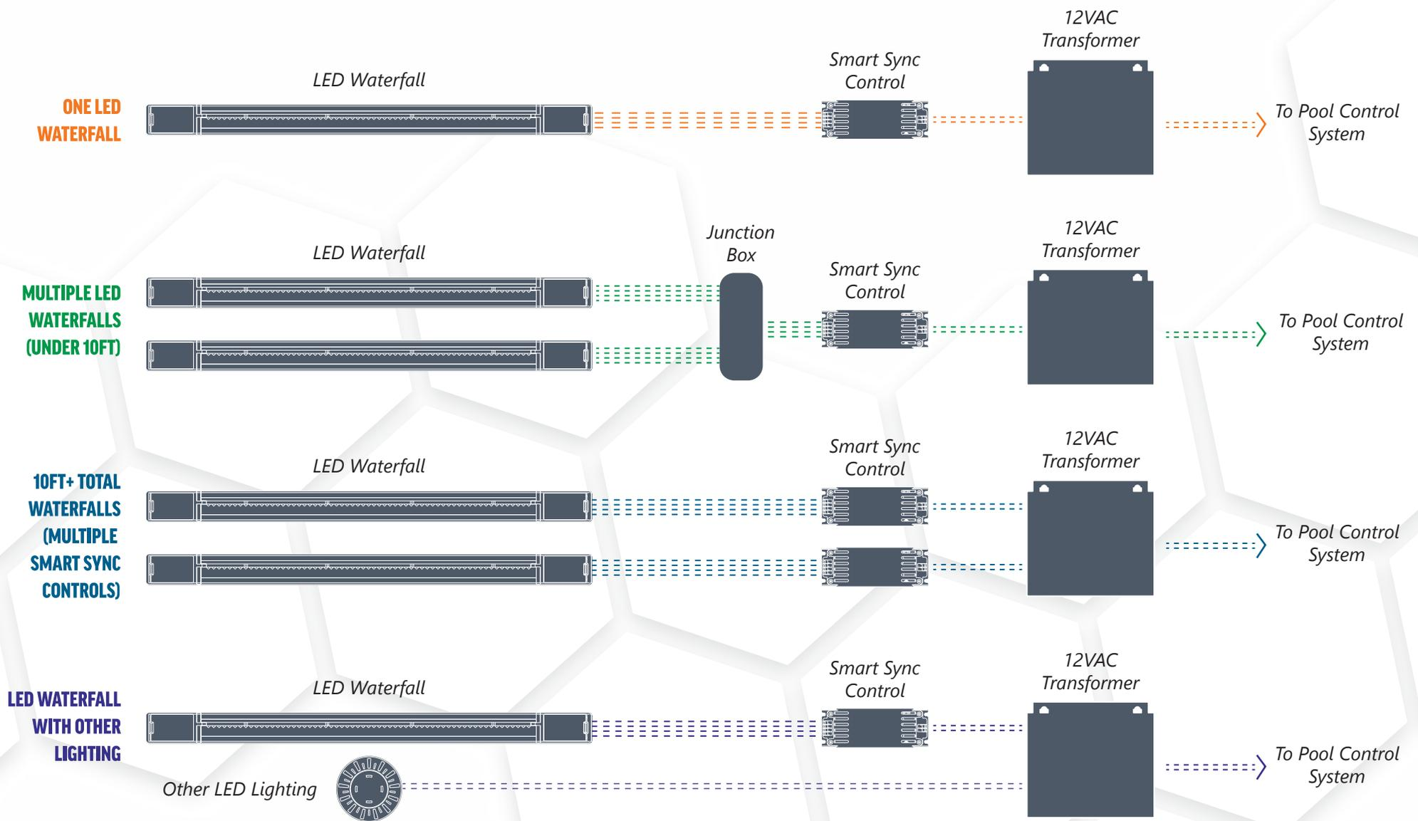
The Smart Sync Control is easy and simple to set up. Simply connect waterfalls to the control, and then to a 12VAC pool transformer. All Smart Sync lighting and compatible controls connected to the same transformer will sync correctly.
