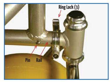
Push back the lever to lock front tire in place.
