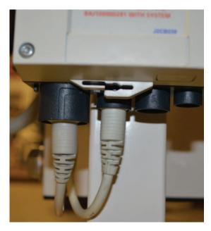
**3.** Apply dielectric grease to the plug terminals.Plug the handset cable
