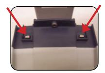
Make sure the contact points of the control box and the battery are not damaged or corroded. If there is corrosion, clean with Scotch-Brite<sup>™</sup> pad. Put some dielectric grease on the contact points before reattaching the battery.
