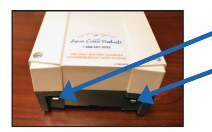
Clean with alcohol and a cotton swab and apply dielectric grease to terminals
