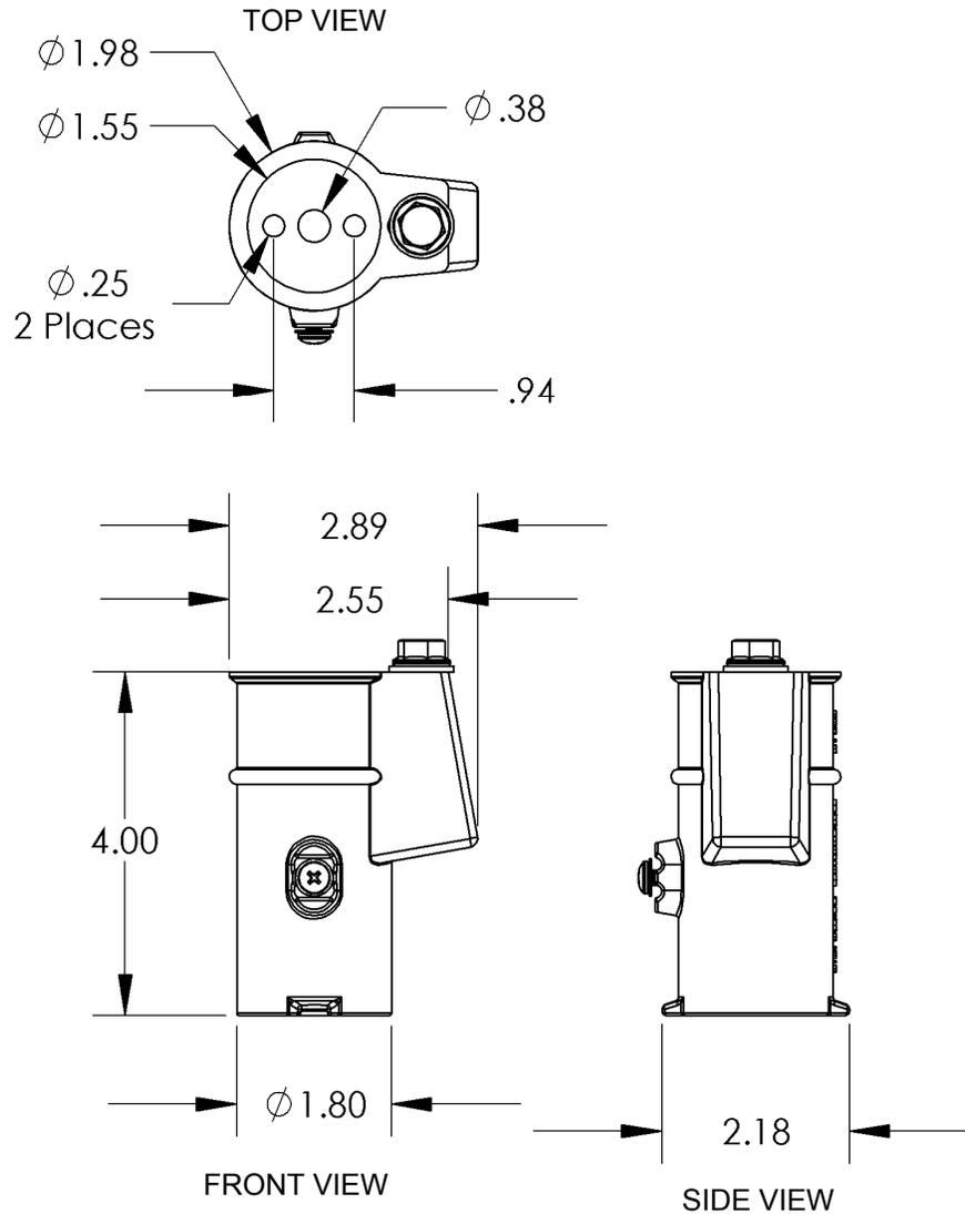
**Specification:** The 1.5" Marine Grade Stainless Steel Anchor Socket assembly includes a 4" (101.6mm) deep cast 316 stainless steel socket and secures fixtures by means of a bronze wedge assembly. The anchor is intended for moderate to heavy-duty commercial use. It is threaded and comes with a #10 UNC brass grounding screw for bonding.
