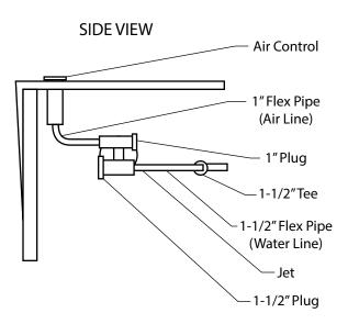
\* Jet assembly is made up of a Body, Wall Fitting, L-Gasket, and a Jet Internal. Install the Jet Internal after plumbing is completed.
