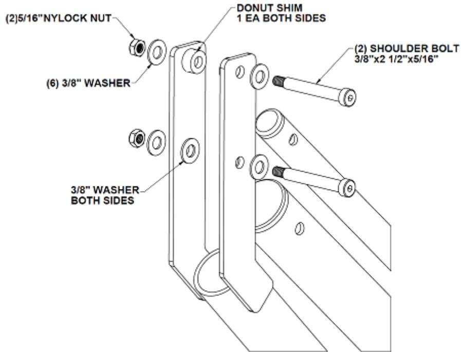
Attach the seat half and the seat belt to the mounting plate of the seat arm using:
