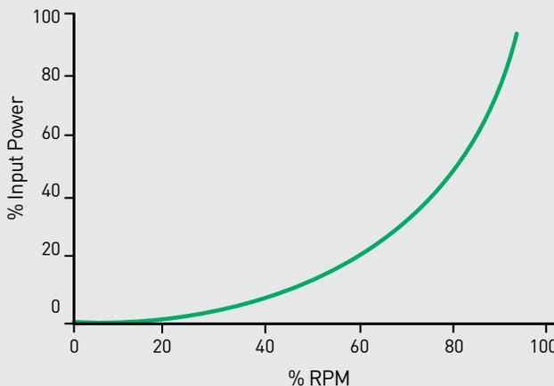
This graph shows the huge increase in energy consumption as pump speed increases. Slow down the pump and you cut energy costs dramatically.
