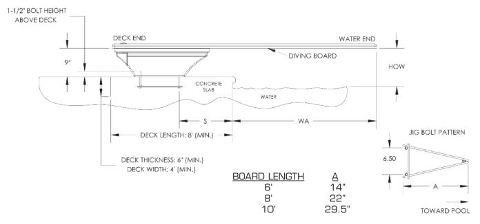
INTER-FAB CANNOT GUARANTEE CUSTOMER'S CONCRETE OR THICKNESS NOTE: WHEN COPING IS USED, DO NOT SET FRONT JIG BOLTS CLOSER THAN 3" FROM THE BACK EDGE OF THE COPING.
