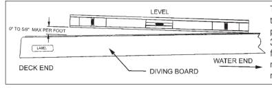
The top surface of the diving board from the deck end to the tip end shall be level or have an upward slope of 5/8" per foot maximum. Elevation difference shall not exceed 3-3/4" (6' Board) or 5" (8' Board) or 6-1/4" (10' Board) from the deck end to the tip of the board. There shall be no downward slope towards the water. The slope shall be measured using a level as shown in the graphic to the left.
