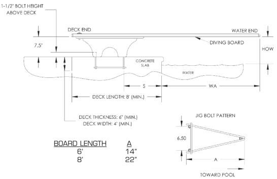
INTER-FAB CANNOT GUARANTEE CUSTOMER'S CONCRETE OR THICKNESS NOTE: WHEN COPING IS USED, DO NOT SET FRONT JIG BOLTS CLOSER THAN 3" FROM THE BACK EDGE OF THE COPING.
