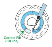
2. Do not over fill the disk. If the disk is overfilled, sample water will flow out of the over flow hole in the center of the disk. The disk is not leaking. Dry the disk and run the test.
